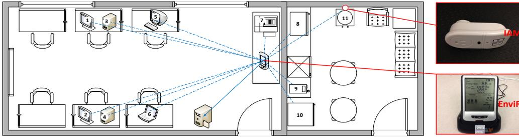
Fig. 2. Energy monitoring platform, monitored appliances, and measuring devices
