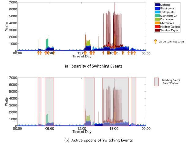
Fig. 1. Energy consumption and appliances' on/off switching events in a house over the course of a day [7]
